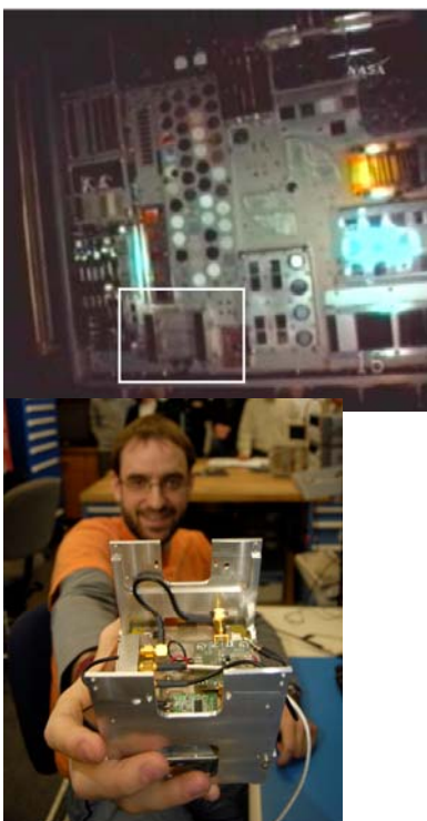
Left: Frame capture of MISSE-6B taken during EVA on March 22, 2008 by astronaut Robert Behnken's helmet video camera upon deployment on the ISS. The white box highlights one of the SSEL designed and built experiments. Bottom: SSEL student engineer holds the Explorer 1 [Prime] satellite.
